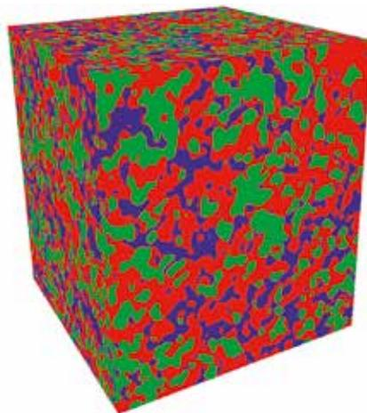
*The method creates a virtual reconstruction of the electrodes' three-dimensional microstructure*
