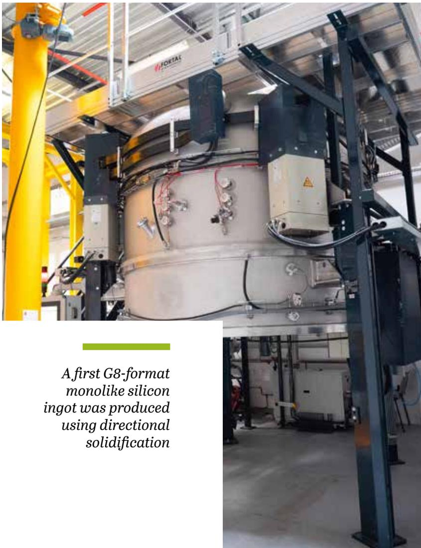
*A first G8-format monolike silicon ingot was produced using directional solidification*
