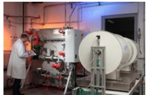
Metal hydride tank designed at CEA TRL 6
